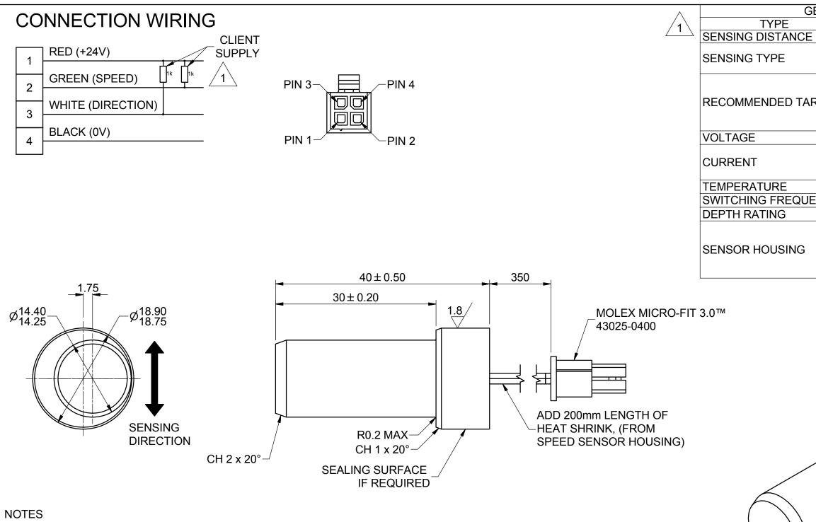
1. SPECIFIATION IS PROVIDED FOR GUIDANCE. FINAL SENSING PARAMETERS AND OPERATION WILL BE DEPENDANT ON MOUNTING ARRANGEMENT AND TARGET DETAILS. TEST ADEQUATELY PRIOR TO FINAL DEPLOYMENT.
